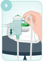
Place nebulizer in cup holder and attach tubing to air inlet on compressor
