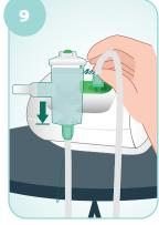
Place nebuliser in cup holder and attach tubing to air inlet on compressor
