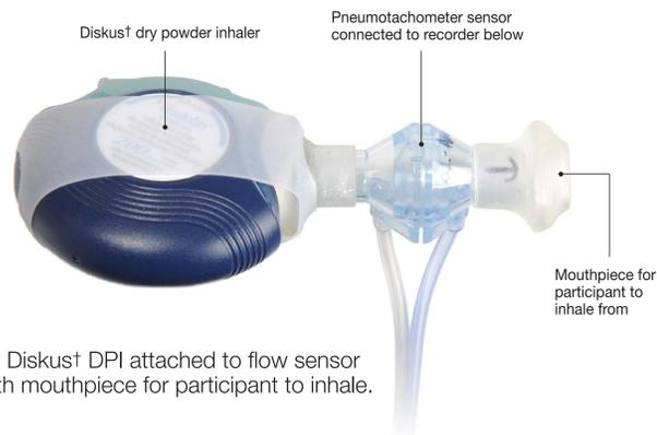
**Figure 1:** Diskus<sup>†</sup> DPI attached to flow sensor holder with mouthpiece for participant to inhale.
