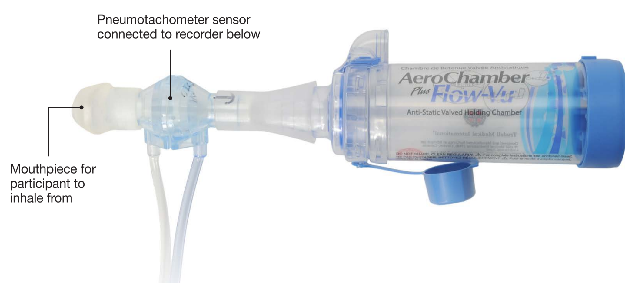
Figure 1: AeroChamber Plus ® Flow-Vu ® VHC attached to flow sensor holder with mouthpiece for participant to inhale.
